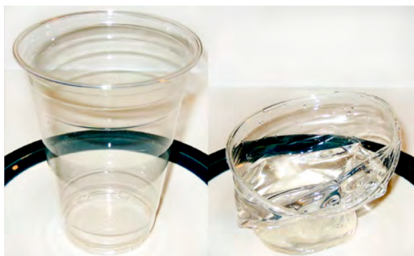
Fig. 2. The effect of hot water on PLA cups – T_g is the glass transition temperature, above which the polymer becomes plastic and returns to its original size.
